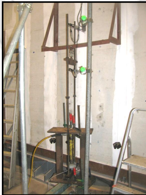
Figure 26: Heavy weight anchorage- wall cupboard
