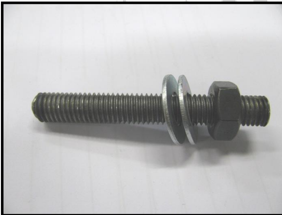
Figure 4: 10mm screw with stainless steel washer – rebar fixz for heavy anchorage test (wall cupboard and wash basin)
