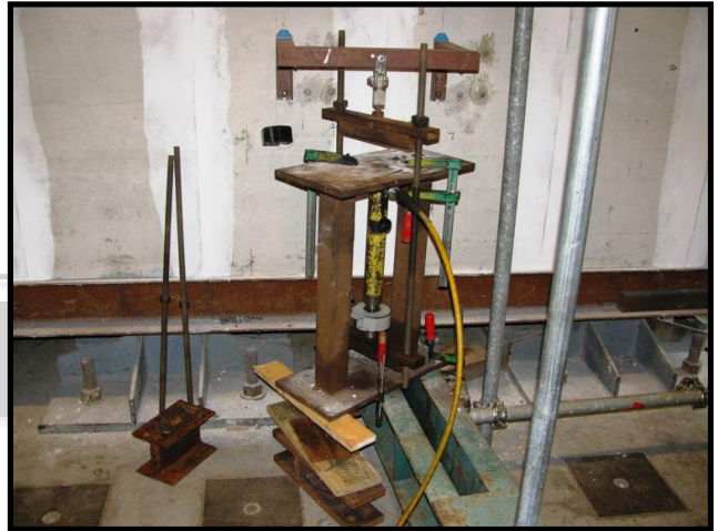
Figure 25: Heavy weight anchorage- wash basin
