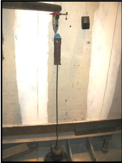
Figure 24: Lightweight anchorage-pull-down test
