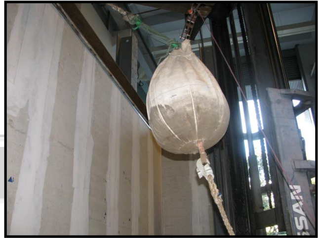
Figure 22: Large soft body impact (resistance to damage / structural damage)
