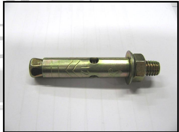
Figure 5: 12mm wallplug with techniglué for heavy anchorage test (wash basin)
