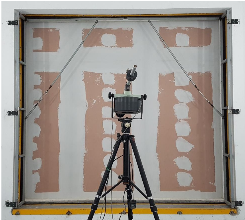
Figure 2 : UAC Acoustic Wall Performance System facing the source room
