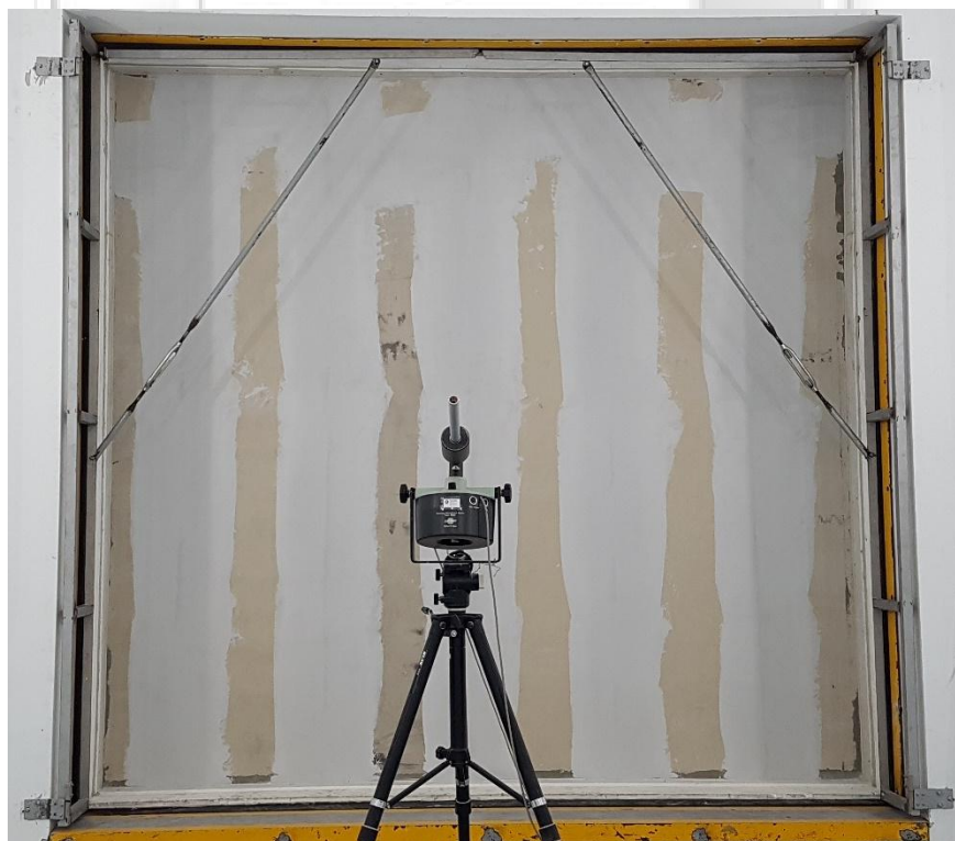
Figure 3 : UAC Acoustic Wall Performance System facing the receiving room
